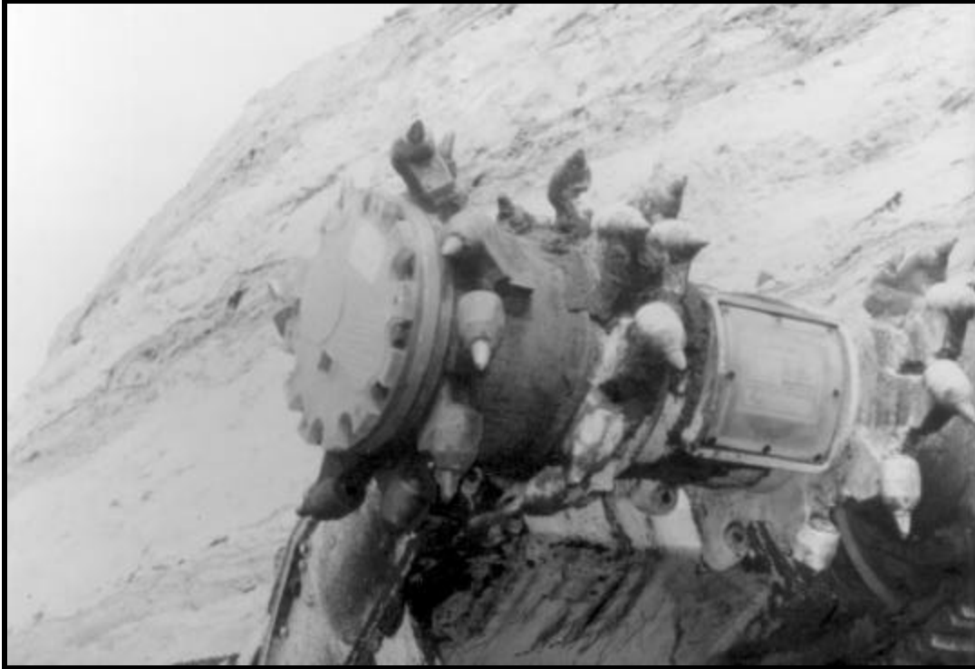
Figure 9. Installation of EDIT horizon sensor on a cutting drum
