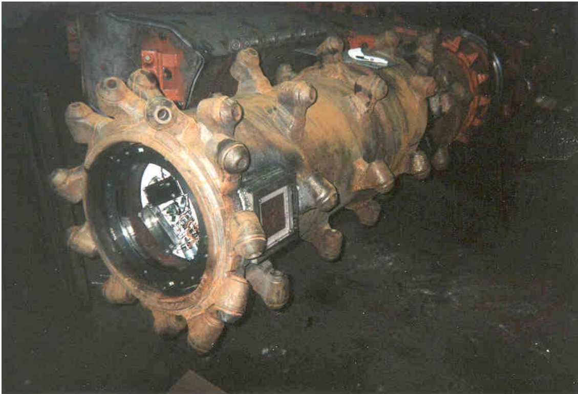
Figure 2. Cutting drum (without bits) with sensor mounted on surface
